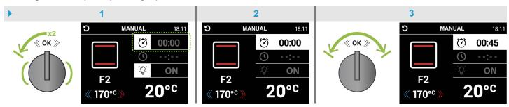
Press the control knob to confirm and exit the selection field (black background, fig. 4), then turn the knob 3 clicks to the right (fig. 5) to exit the setting (and the icons 3 illuminated in sequence) to avoid entering the TARGET TEMPERATURE modification field.
