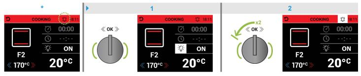
In the MINUTE MINDER screen, the "HOURS/h" field is already active (white background, fig. 3) and can be **set** by turning the **control knob** within **10 seconds** several clicks to the **right** or **left** to increase or decrease the **value**; **press** the knob to switch to the "MINUTES/m" field (fig. 4) to set the **value** as described above. Then **press** the knob to confirm and return to the **COOKING** screen. The icon will be active (fig. 5) and the programmed countdown **begins**.
